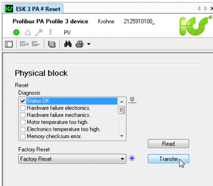
The reset function is selected and transferred, upon which the diagnostics of the field device is updated.
