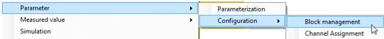
The block management can be used to configure the quantity and the numbers of the transducer and function blocks of a profile DTM. A new copy of an existing block, including its parameters, can be generated in addition.
